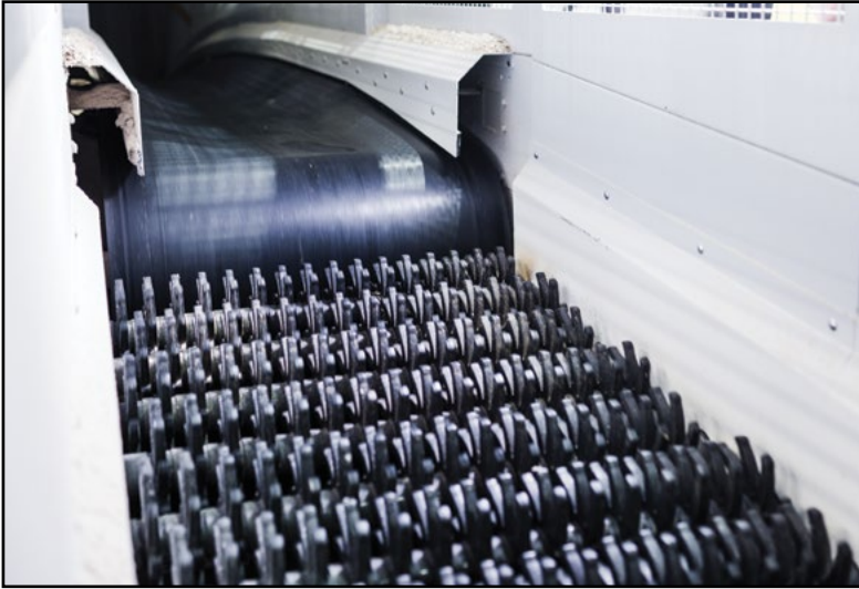
The star screening machine separates excess lengths from the material.
