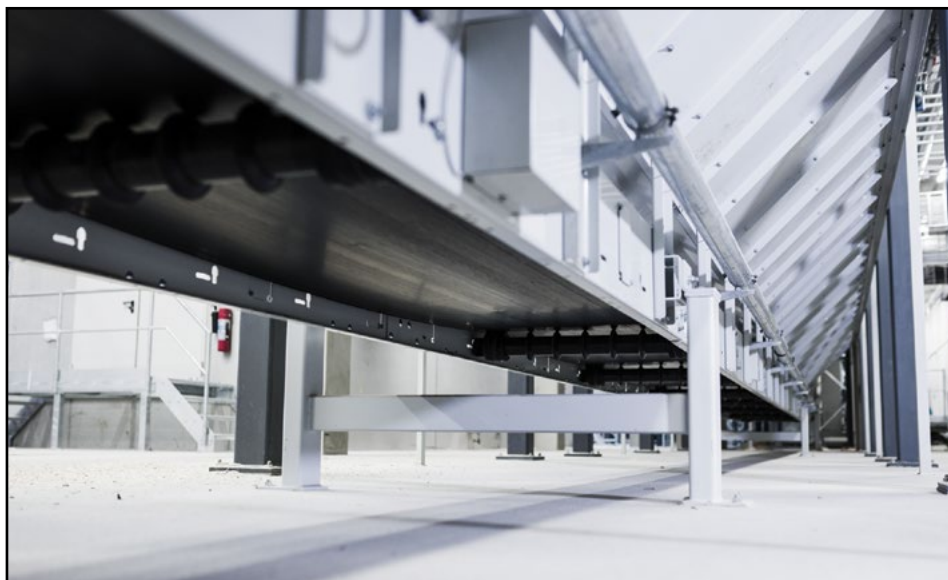
The waste wood falls directly from the sawmill on to the conveyor system, ready for the next stage of pellet production.
