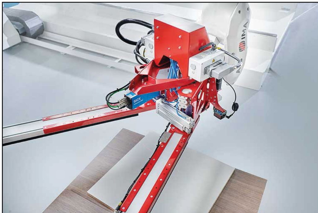
Innovation at LIGNA: IMA Schelling has developed an automated handling system for its fh4 and fh5 panel-sizing saws.
