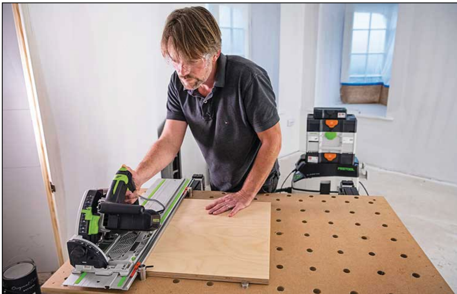
Tim Styles using a track saw cutting station made using the UJK Parf MKII guide system.
