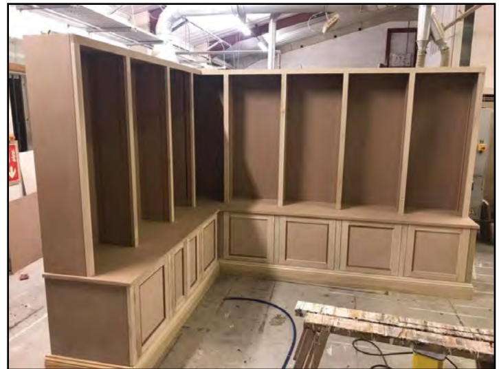
A mix of MDF and hardwoods for this bookcase ready for painting and fitting.
