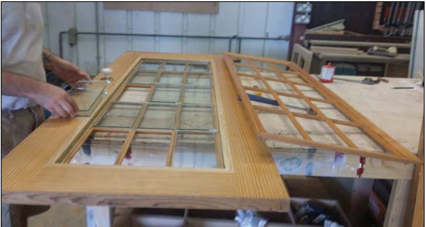
Multi-pane glazed internal doors make up a good proportion of the work undertaken in the company's workshops.
