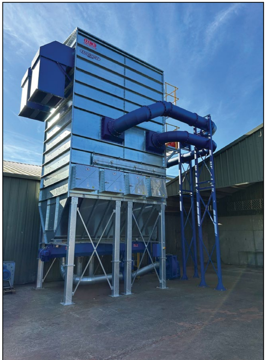
The DCE Envirojet W-Series ensures highly efficient dust extraction across processing areas, maintaining clean, healthy air for workers.
