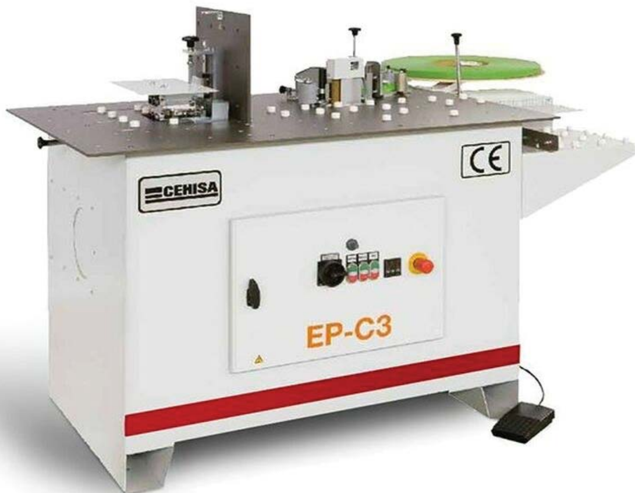
The Cehisa EP-C3 is a hot-melt, compact, semi-automatic edge-bander for internal and external radius curved work.
